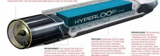
**AIR BEARINGS** The capsule will ride on a cushion of air pushed from the bottom of launch-tray-size sleds. Landing gear may need to be deployed as it comes to a stop.
