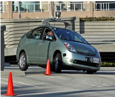
The Google driverless car is powered by artificial intelligence that utilizes the input from the video cameras inside the car, a sensor on the vehicle's top, and some radar and position sensors attached to different positions of the car. Sounds like a lot of effort to mimic the human intelligence in a car, but so far the system has successfully driven 1609 kilometers without human commands.
