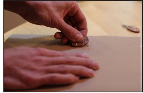
Step 9: Starting with your coarsest sandpaper, sand down the surfaces of your wood pieces until reasonably smooth. Place the sandpaper face up on a flat surface and rub the block across the paper rather than sanding from above. Once the surface is flat, polish out the remaining scratches with fine-grit sandpaper. The lead from your pencils may smear across the surface during sanding, but you can remove any stray marks with an eraser or with careful sanding of the stain.
