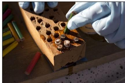
Step 8: Retrieve your block. Peel the masking tape off of the back and make absolutely sure the epoxy is dry before continuing. It's now time to cut the block into thinner sheets. First, cut off any pencil ends that stick out. Next, draw a line down the side of the block, approximately 1/8" from the top, and carefully cut off a sheet by following this line
