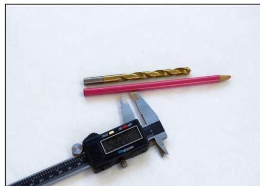
Step 2: Find a drill bit that roughly matches the size of the pencils. We used a fancy caliper, but use a ruler or even just hold the two up to each other to compare.
